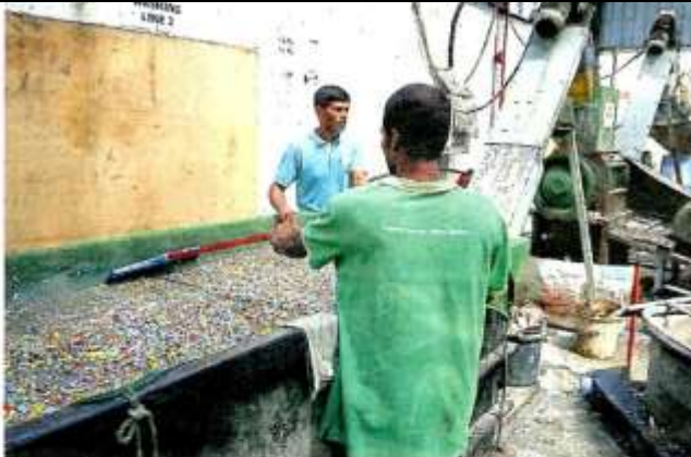
Valuable junk: Workers sorting out the plastic waste before it undergoes several processes to be made into plastic resin, which is then used to manufacture new products.
